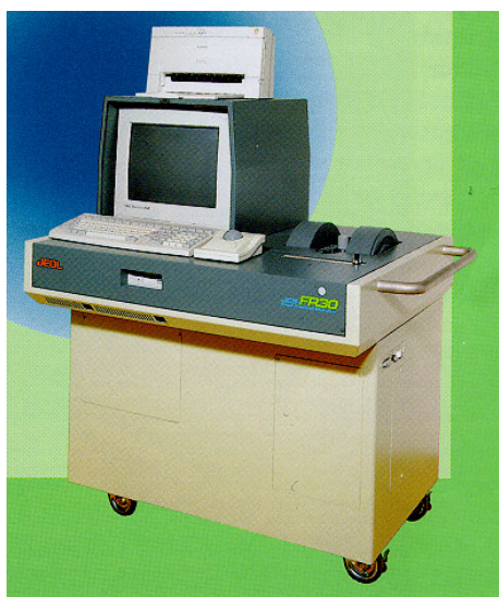
Figure 7: Photo of the mobile JEOL FR30 EPR instrument for detecting free radicals in blood samples. EPR spectrum of the ascorbyl radical in human plasma.
